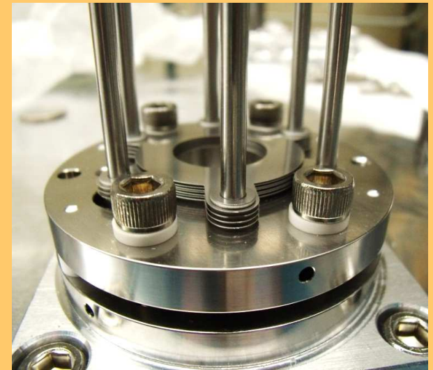
2 electrically insulated stacks
