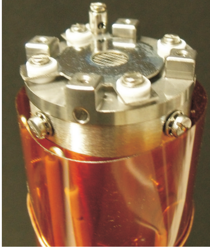
Figure C.11: Picture of the RGS head without ion source. The leads that connected to the ion source were bent backwards and are electrically isolated by a Kapton foil. The lens with the mesh at the center of the picture is biased at -115\text{ V} with respect to ground.
